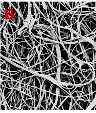
Photograph B opposite is a cross section of a less expensive screen cleaning roll sourced in the Far East which is resin bonded, which means that a type of glue has been used to bond the fibres together.
