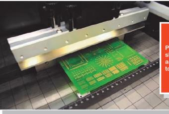
PCB on printing table showing locating arrangement on tooling rails.
